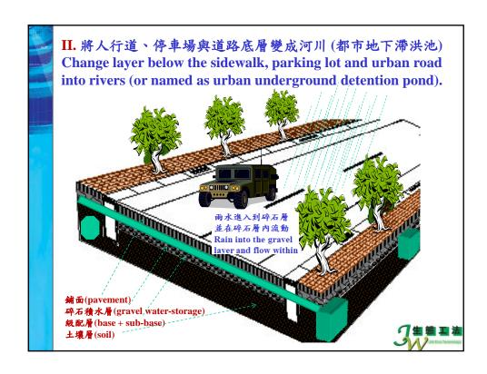
透水鋪面兩水渗透率 permeability of permeable pavement:
